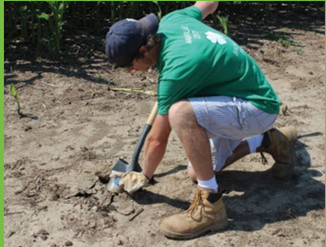
Collection of soil core samples for determination of plant-available air and water capacities.
